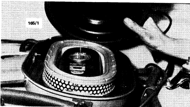
The air cleaner element should be renewed at the recommended intervals.
