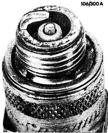
Spark plug with burnt electrodes and white blistered appearance. Possibly due to incorrect plug type, loose plug or motor running too hot.
