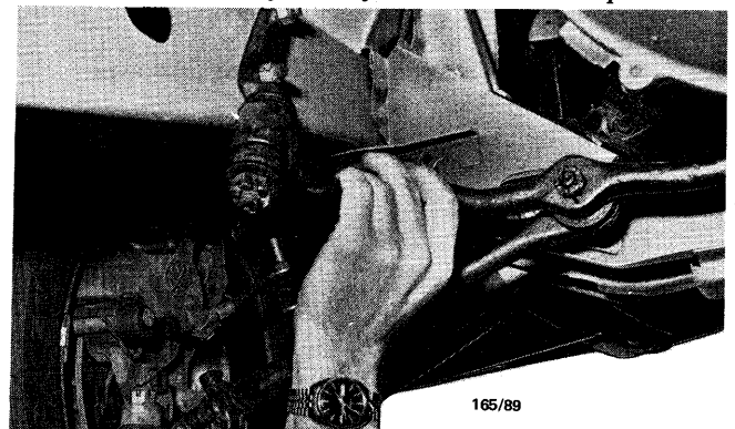
Checking idler arm assembly for wear.
