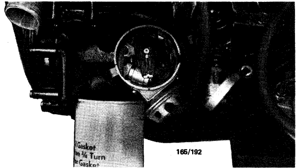
Rotor pointing to No 1 cylinder position on distributor.
