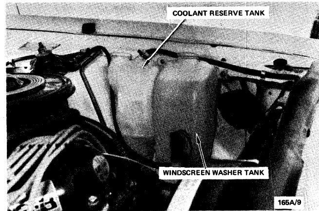
View of coolant reserve tank installed in vehicle.
