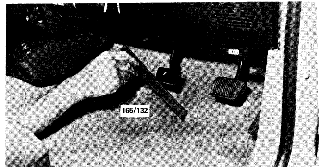
Check and adjust clutch pedal height.
